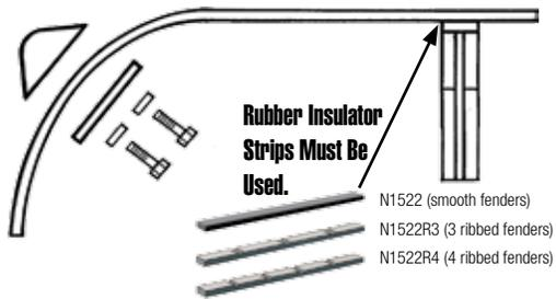
4. The fenders must be positioned so that they are aligned properly. This means that all surfaces must make contact with the brackets without the fender requiring any twisting or bending. Should the fender require twisting to attach it to the brackets, you risk premature unwarranted failure.
